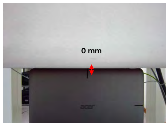
Fig.5 EUT Secondary Landscape mode to flat phantom
