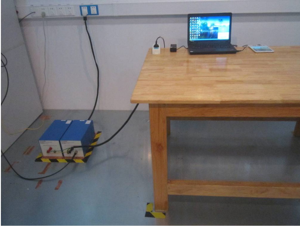
Conducted Emissions Test Setup Front View
