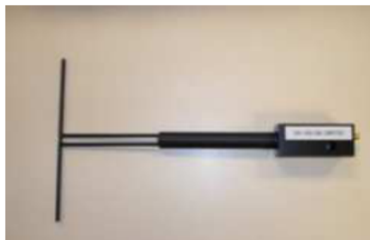
Figure 1 – Satimo COMOSAR Validation Dipole
