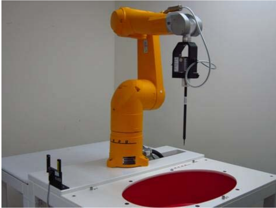
Fig.1 Photograph of the SAR measurement system
