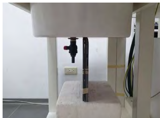
Fig.5 EUT Bottom side to flat phantom
