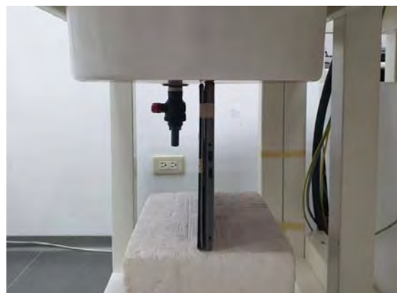
Fig.4 EUT Top side to flat phantom
