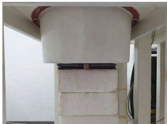
Fig.3 EUT Back side to flat phantom
