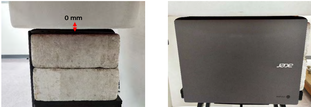
Fig.3 EUT Bottom side to flat phantom
