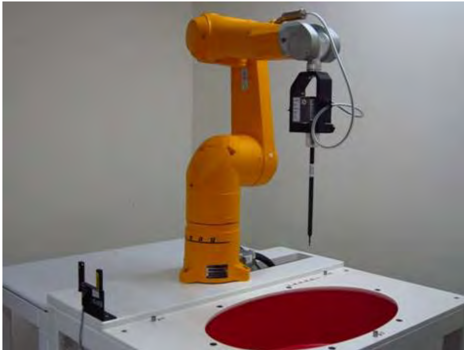
Fig.1 Photograph of the SAR measurement system
