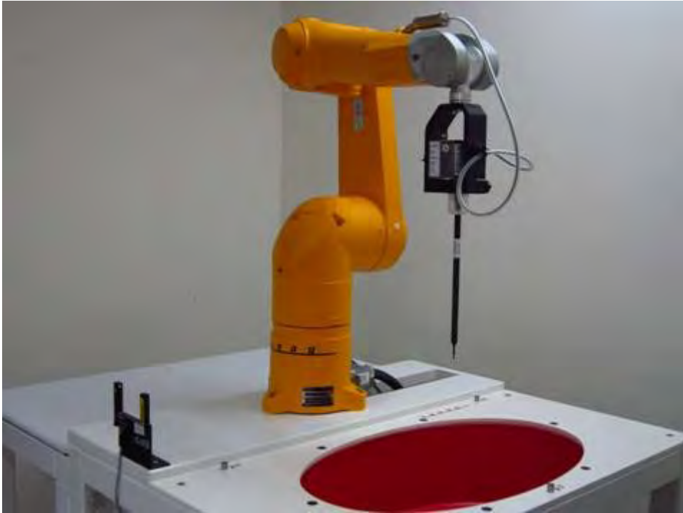
Fig.1 Photograph of the SAR measurement system
