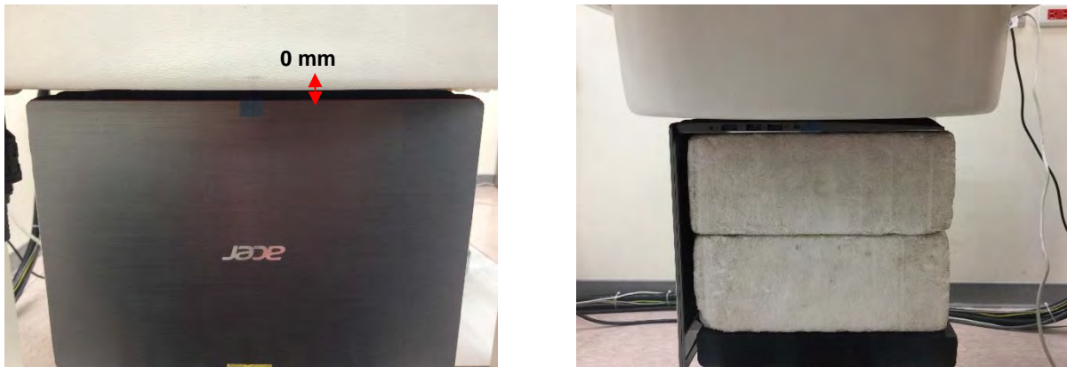
Fig.3 EUT Bottom side to flat phantom
