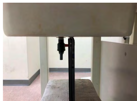
Fig.5 EUT Bottom side to flat phantom
