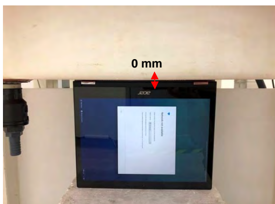
Fig.5 EUT Bottom side to flat phantom
