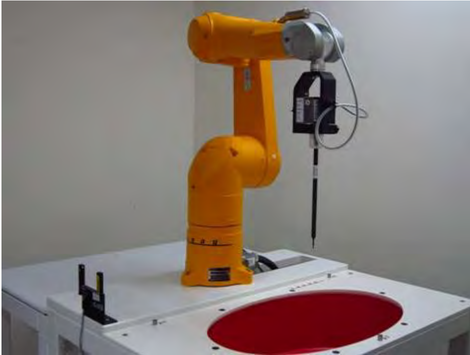
Fig.1 Photograph of the SAR measurement system
