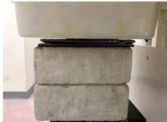
Fig.3 EUT Back side to flat phantom
