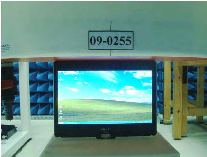
Figure 1. Body SAR Test Setup (Flat Section)_ Tablet Mode LCD Tip Close Body
