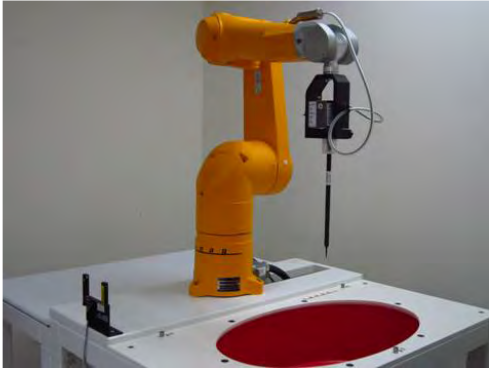
Fig.1 Photograph of the SAR measurement system
