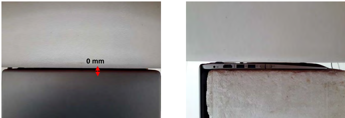
Fig.3 EUT Back side to flat phantom
