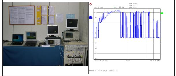
EUT (Client) links with master on 5510MHz
