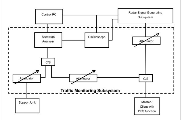
The test transmission will always be from the Master Device to the Client Device. While the Client device is set up to associate with the Master device and play the MPEG file (6 y Magic Hours) from Master device, the designated MPEG test file and instructions are located at: <a href="http://ntiacsd.ntia.doc.gov/dfs/">http://ntiacsd.ntia.doc.gov/dfs/</a>.
