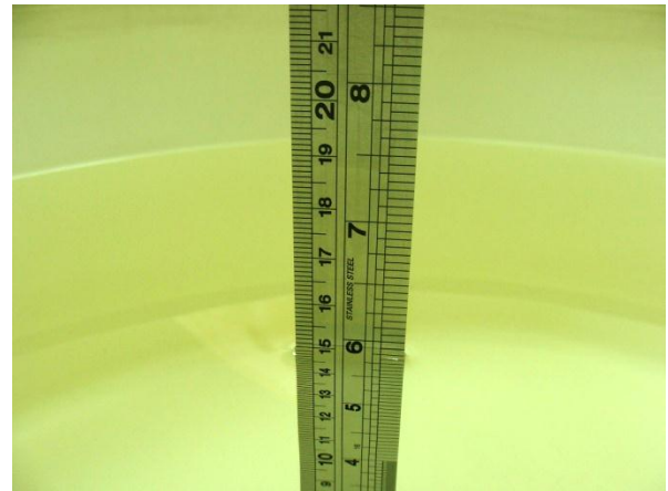
Fig 6.2 Photo of Liquid Height for Body SAR
