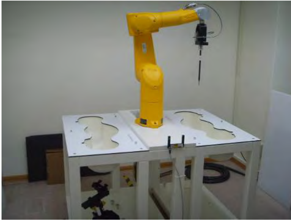
Fig.1 Photograph of the SAR measurement System
