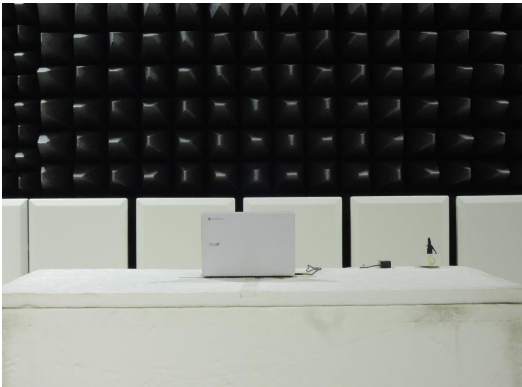
Radiated Emission Set up Photos (Front View)
