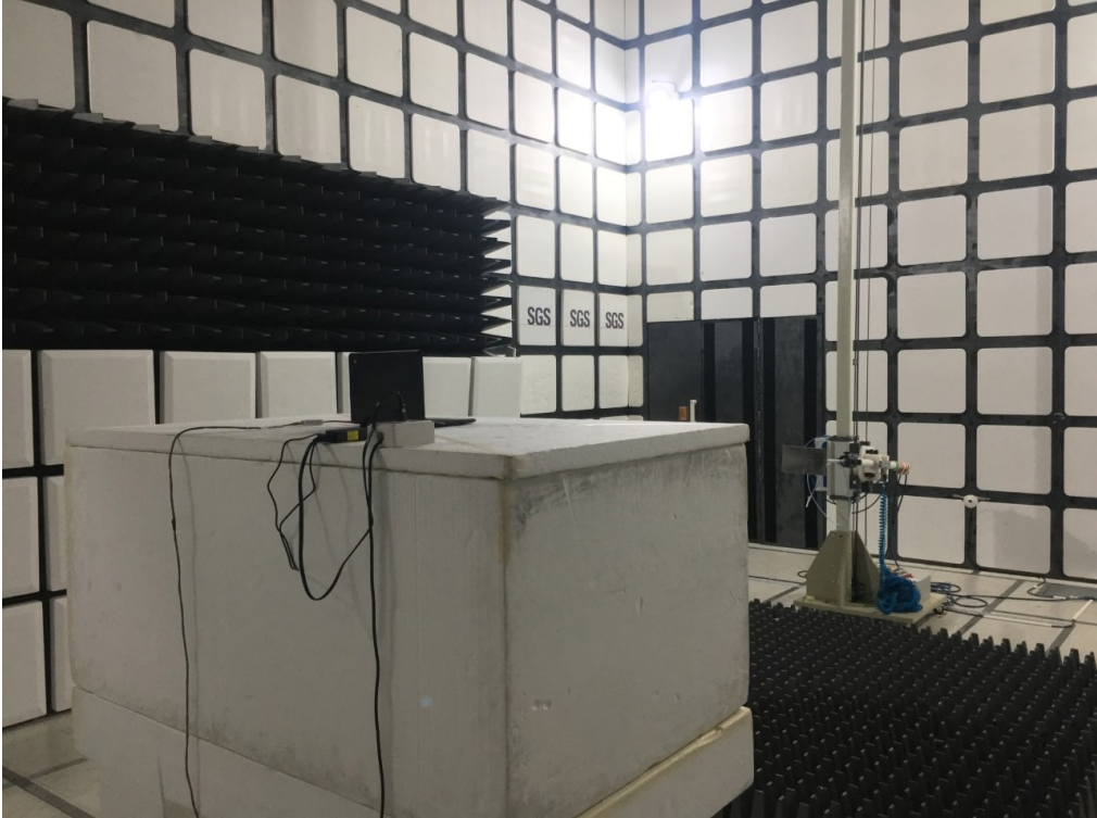
Radiated Emission Set up Photos (Above 1GHz)
