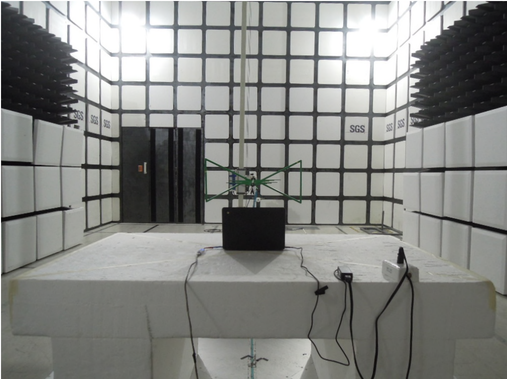
Radiated Emission Set up Photos (Above 1GHz)
