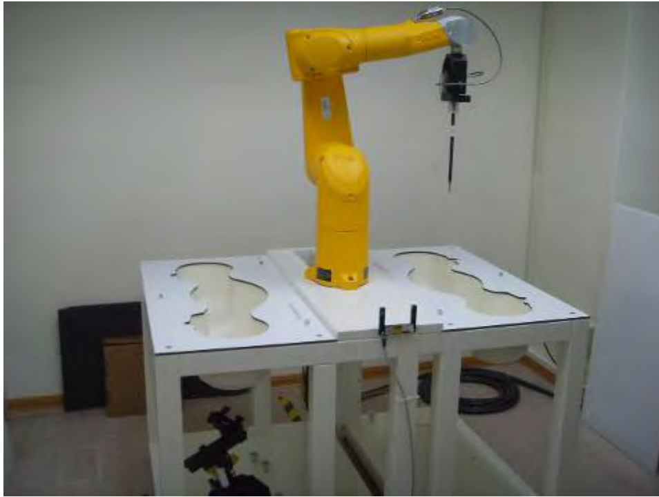
Fig.1 Photograph of the SAR measurement System
