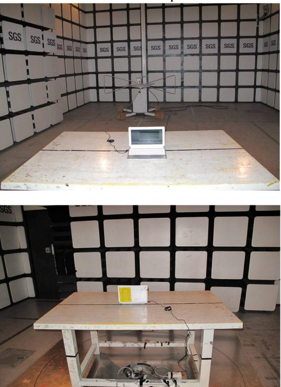
**Radiated Emission Set up Photos**
