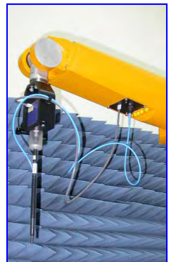
Figure 4. Probe setup on robot
