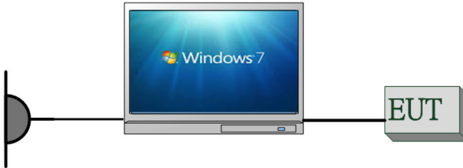
Fig. 2-2 Conduction (AC Power Line) Configuration
