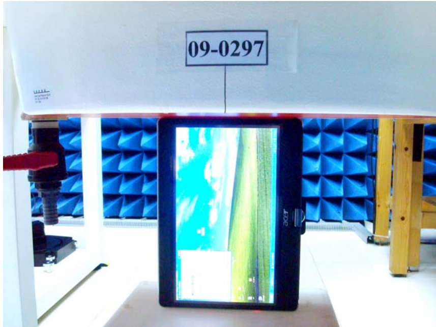
Figure 3. Body SAR Test Setup (Flat Section)_ Tablet Mode LCD Right side Close Body
