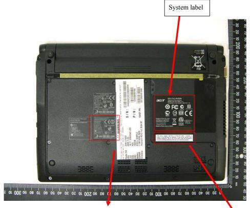
Partial label, indicate "This device contains WLAN module Atheros AR5B95"
