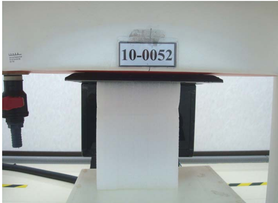
Figure 1. Body SAR Test Setup (Flat Section) Host: LCD Open 90° Bottom Close Body
