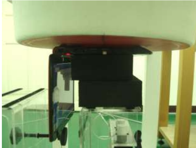
Bottom of the Laptop with Phantom 0 cm Gap
