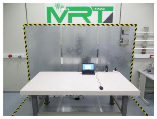
Test Mode 3 Description: Back View of Conducted Emission Test Setup
