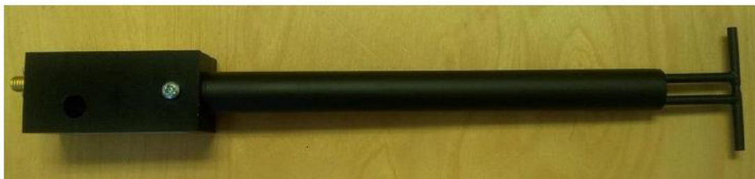
Figure 1 – MVG COMOSAR Validation Dipole
