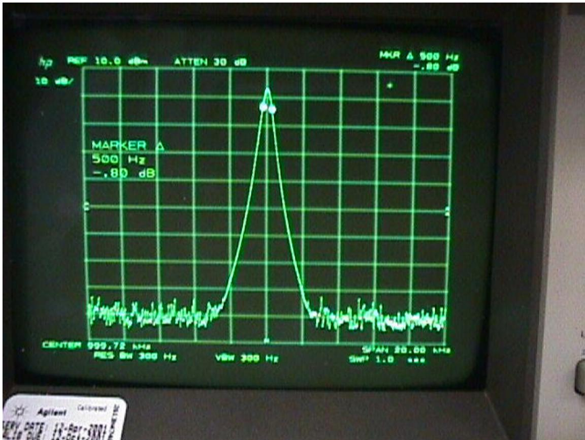
The 6 dB bandwidth is seen to be 500 Hz. The 20 dB bandwidth can be seen to be approximately 3 kHz.
