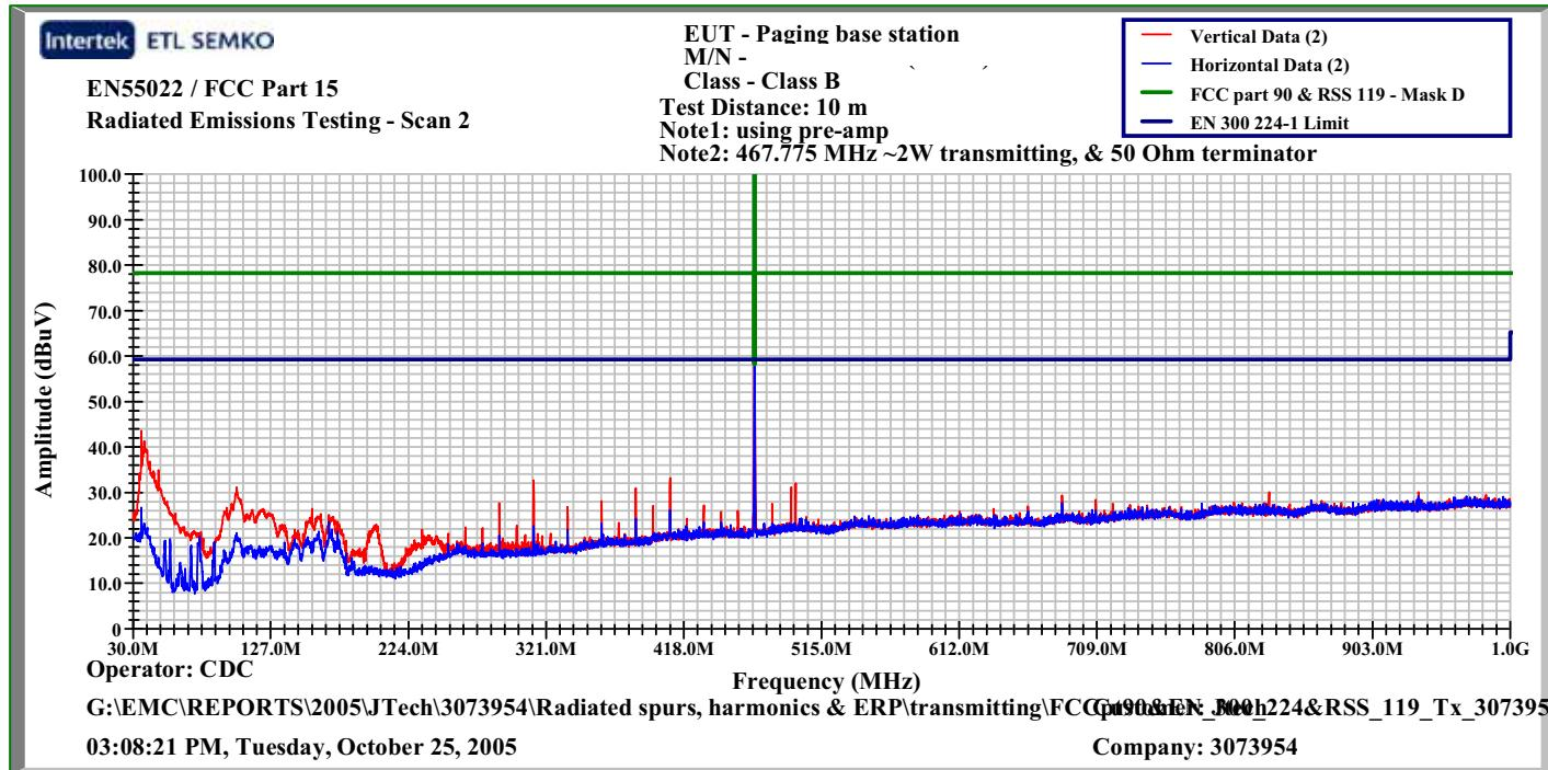
Transmitter Radiated Spurious Emissions Results
