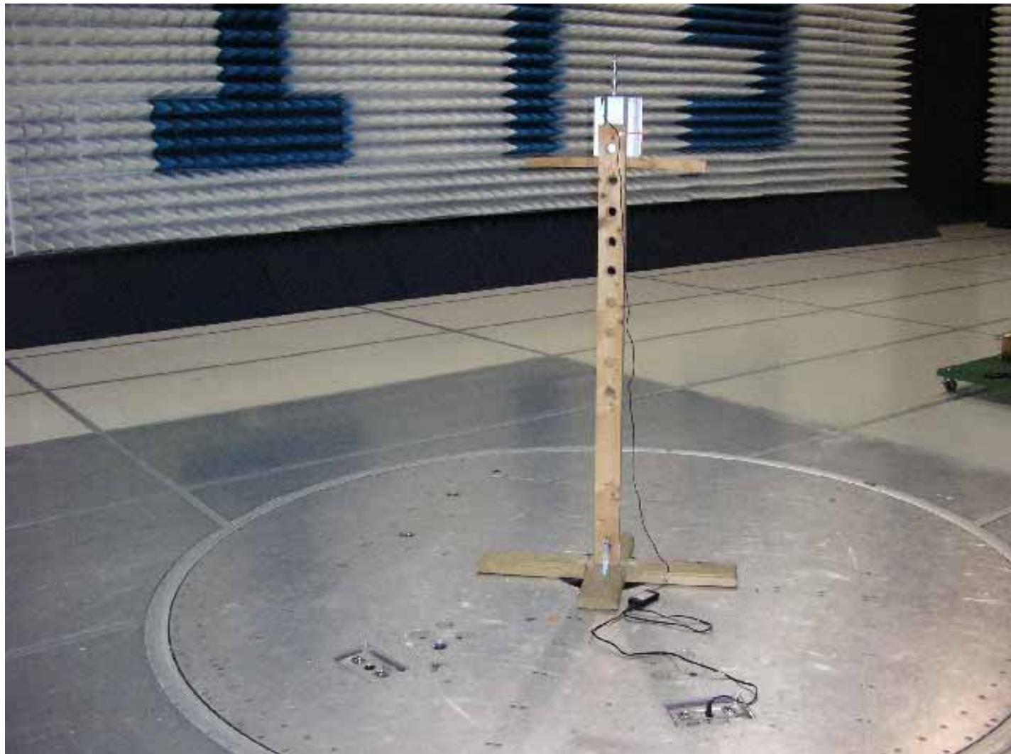
Radiated Spurious Emissions Test Setup
