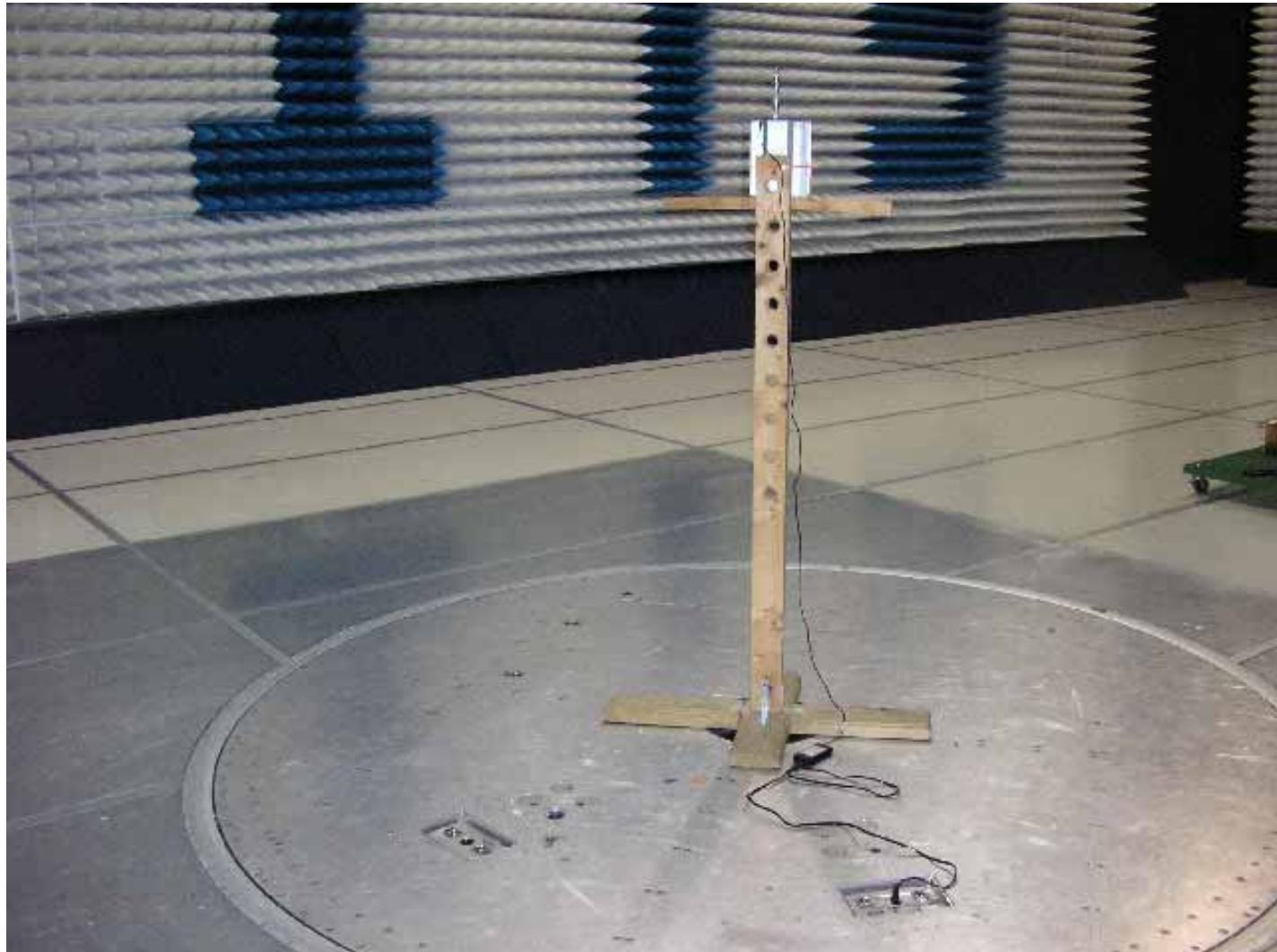
Radiated Spurious Emissions Test Setup
