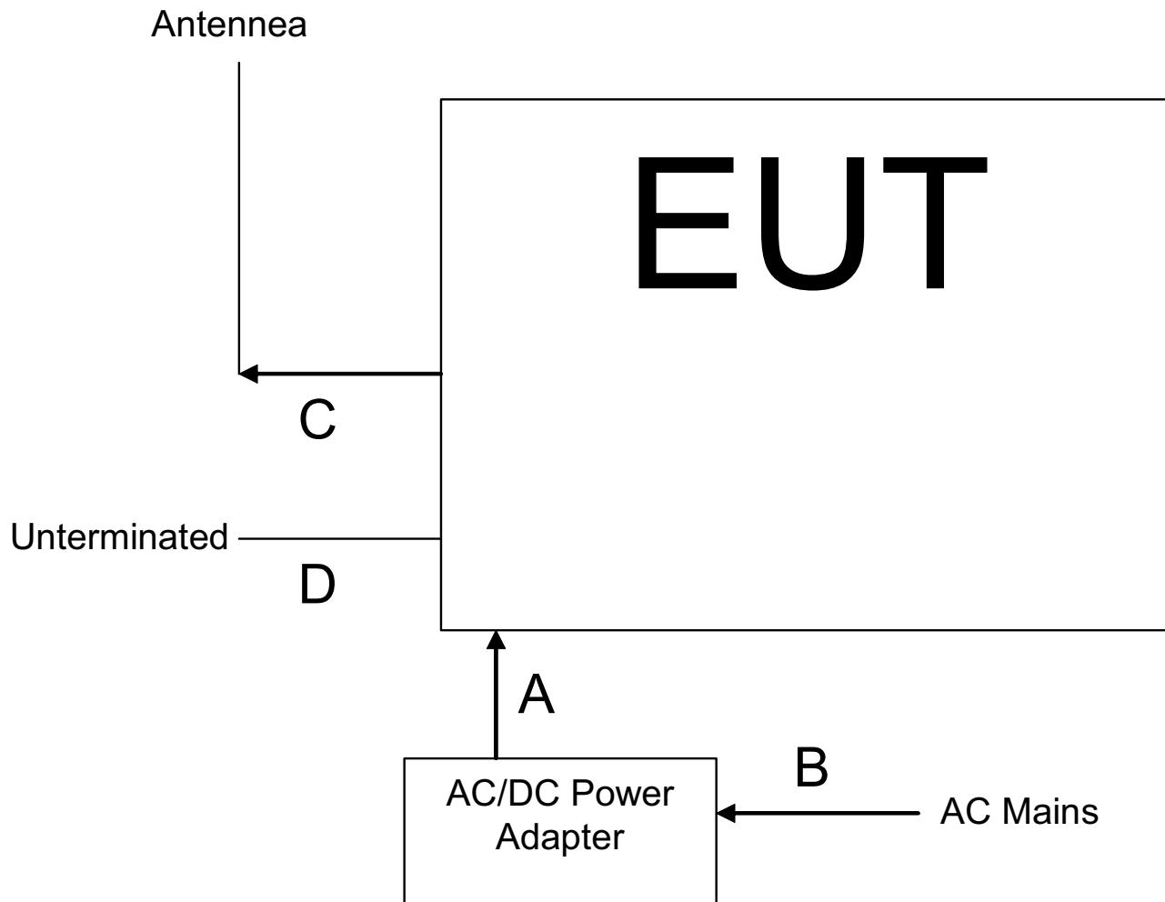
Cable Interconnection &amp; Support Equipment Diagram
