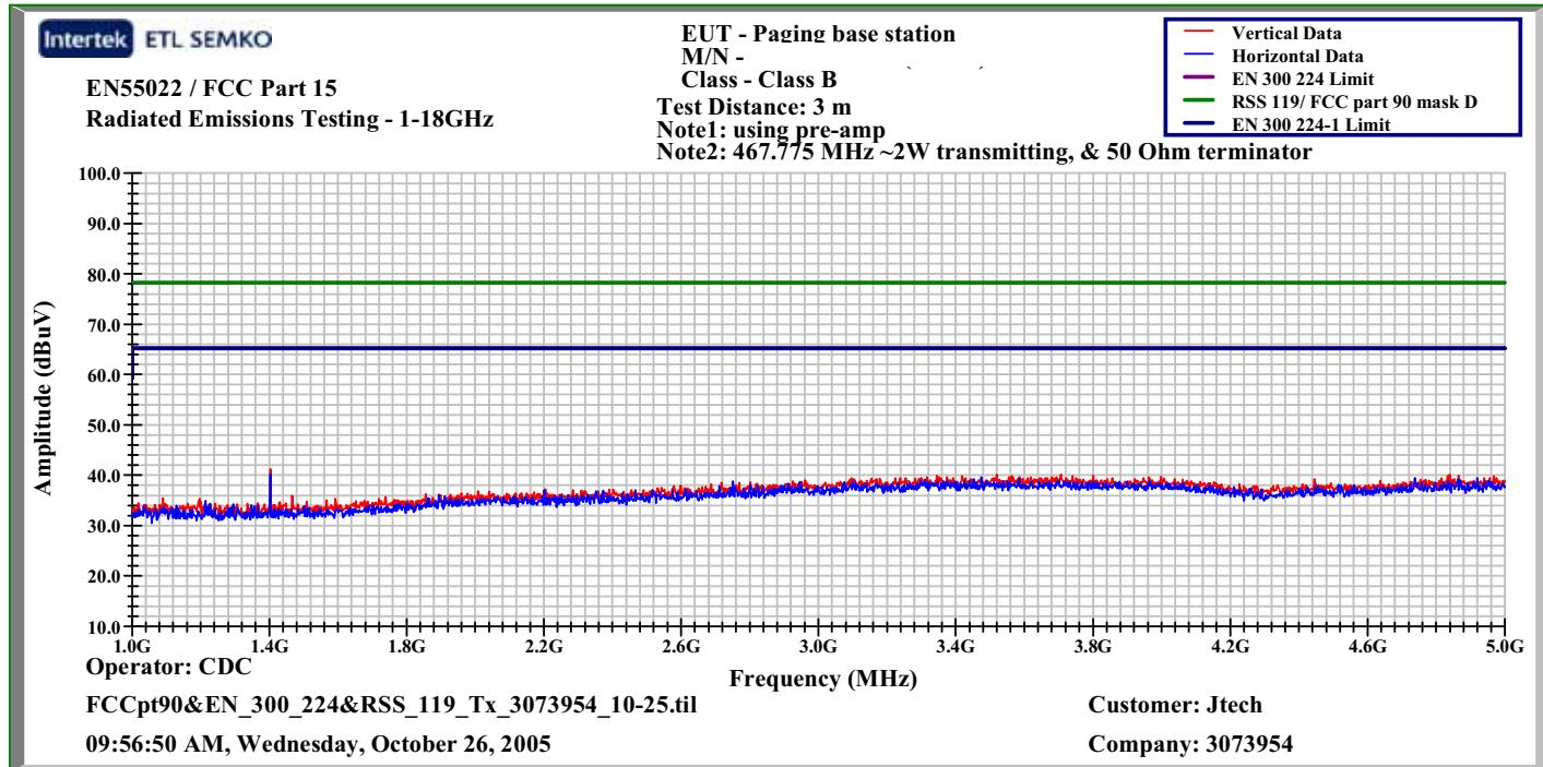
Transmitter Radiated Spurious Emissions Results
