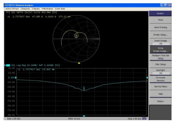
D1750V2, serial No. 1108 Extended Dipole Calibrations
