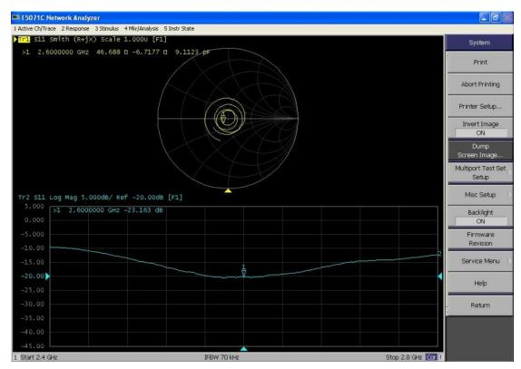
D2600V2, serial No. 1074 Extended Dipole Calibrations
