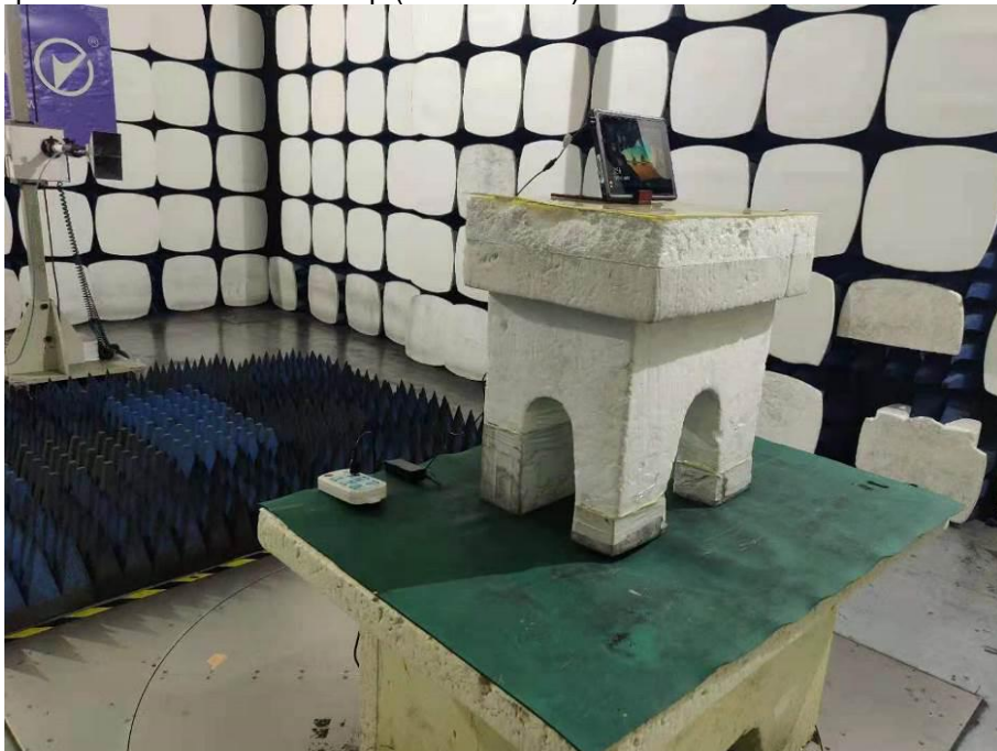
Spurious Emission Test Setup (Above 1GHz)
