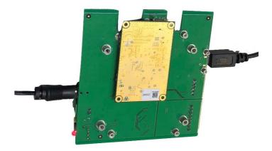
5. Insert the connector of antenna into the antenna port of the RM100 UHF RFIDReader Module.
