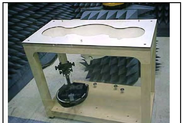
Figure 6. SAM Twin Phantom
