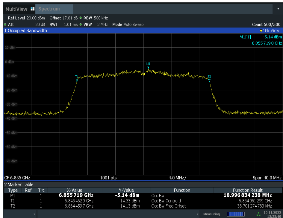
Fig.53 99% Occupied Bandwidth (802.11ax-HE20, 6855MHz)
