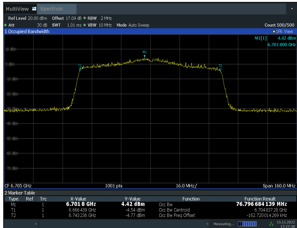
Fig.77 99% Occupied Bandwidth (802. 11ax-HE80, 6705MHz)
