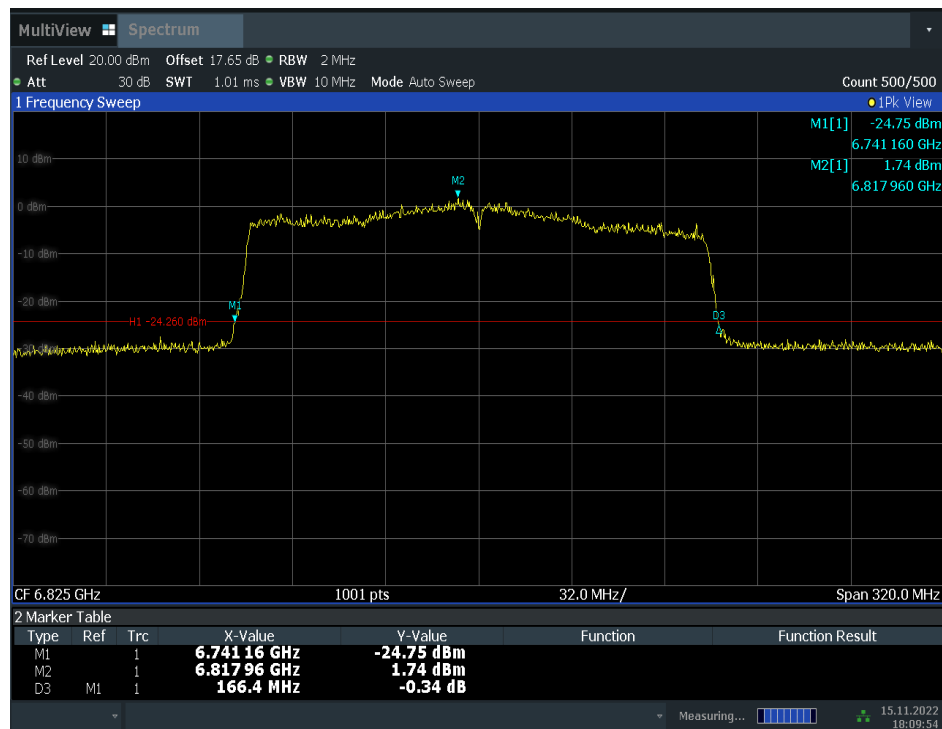
Fig.43 Occupied 26dB Bandwidth (802. 11ax-HE160, 6825MHz)
