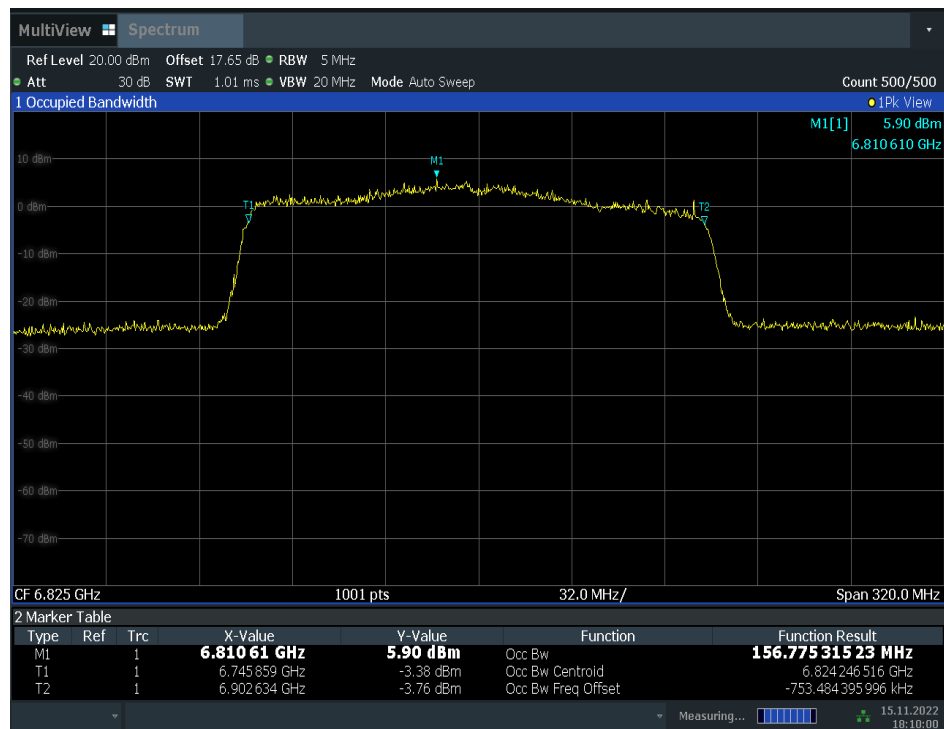
Fig.87 99% Occupied Bandwidth (802. 11ax-HE160, 6825MHz)
