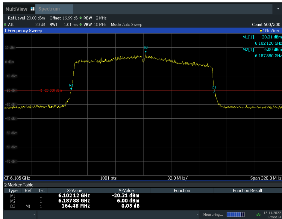
Fig.39 Occupied 26dB Bandwidth (802. 11ax-HE160, 6185MHz)
