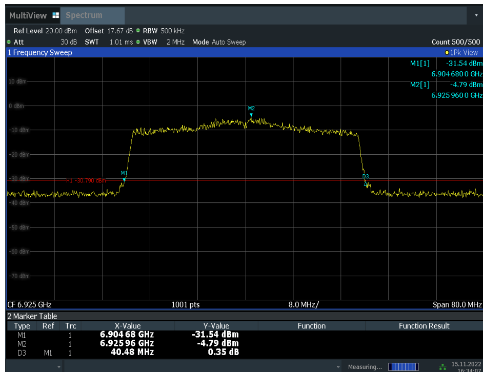
Fig.24 Occupied 26dB Bandwidth (802.11ax-HE40, 6925MHz)
