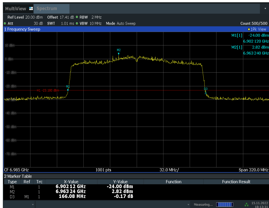
Fig.44 Occupied 26dB Bandwidth (802. 11ax-HE160 6985MHz)
