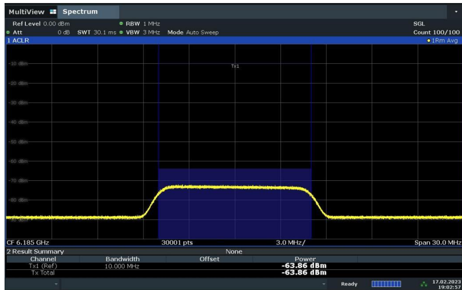
Fig.91 AWGN Signal Level 802.11ax HE160 6185 (middle, at Antenna Port)
