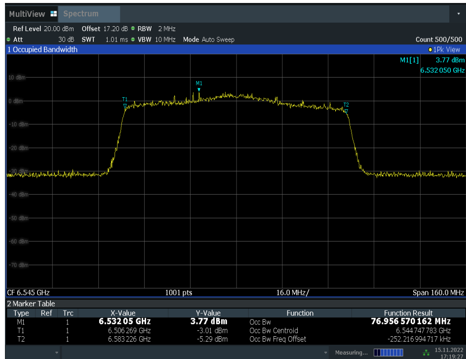
Fig.75 99% Occupied Bandwidth (802. 11ax-HE80, 6545MHz)
