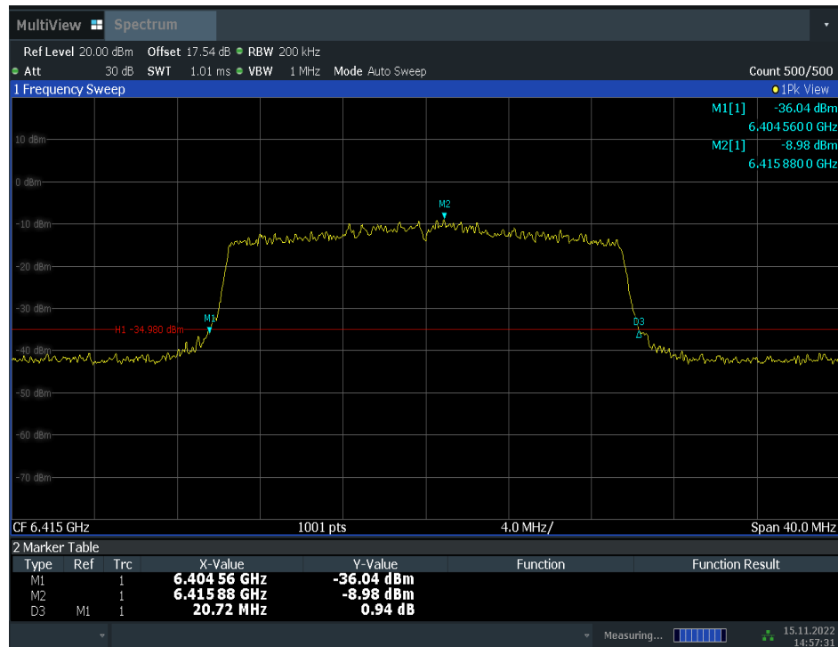
Fig.3 Occupied 26dB Bandwidth (802.11ax-HE20, 6415MHz)
