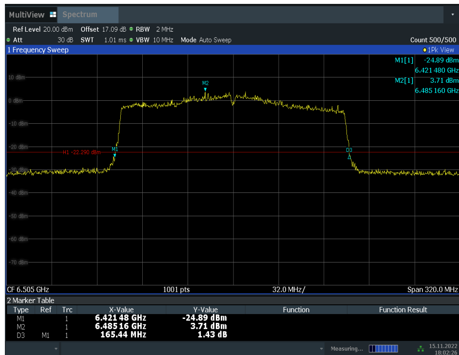
Fig.41 Occupied 26dB Bandwidth (802. 11ax-HE160, 6505MHz)
