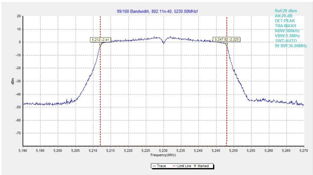
Fig. 40 99% Occupied Bandwidth (802.11n-HT40, 5230MHz)
