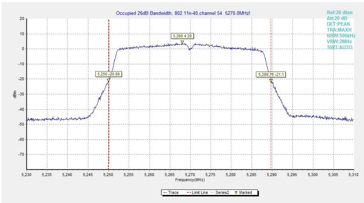
Fig. 12 Occupied 26dB Bandwidth (802.11n-HT40, 5270MHz)
