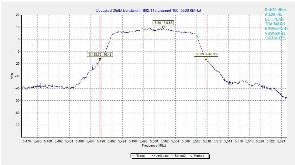
Fig. 7 Occupied 26dB Bandwidth (802.11a, 5500MHz)
