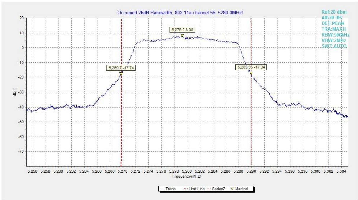
Fig. 5 Occupied 26dB Bandwidth (802.11a, 5280MHz)
