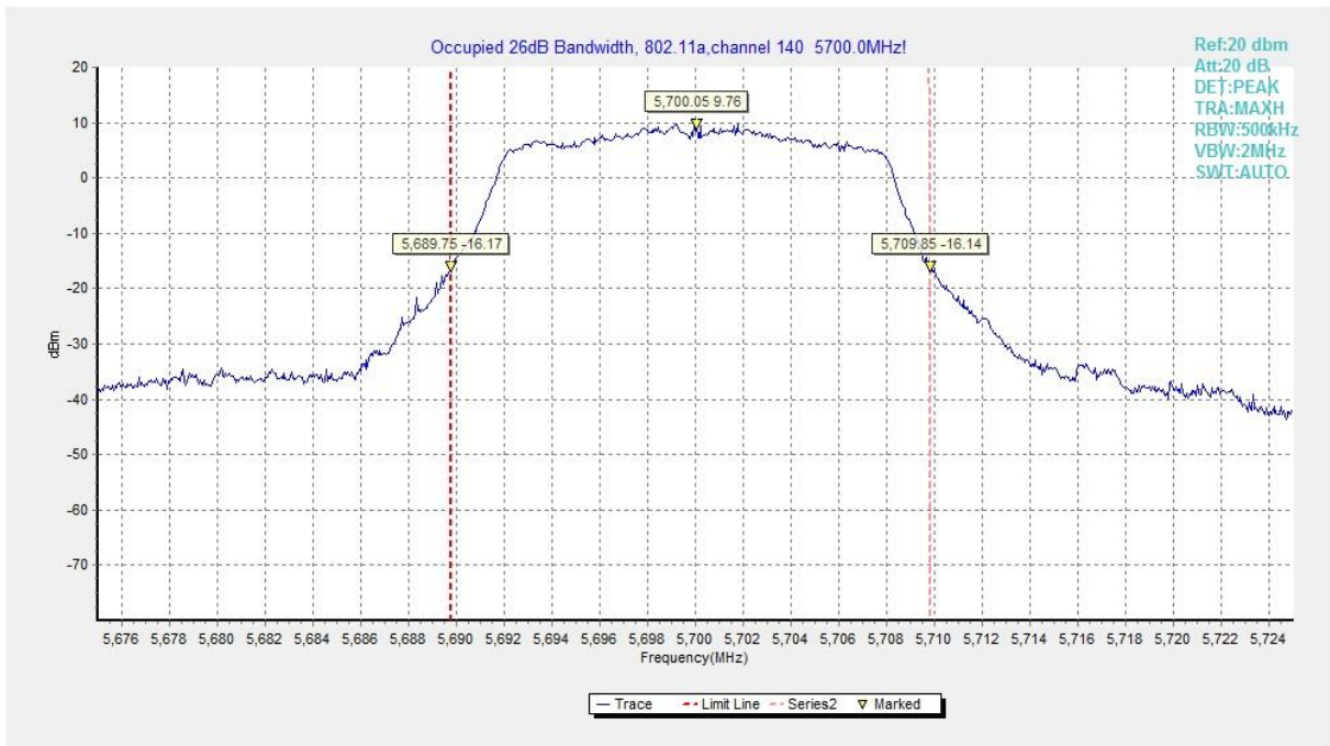
Fig. 9 Occupied 26dB Bandwidth (802.11a, 5700MHz)
