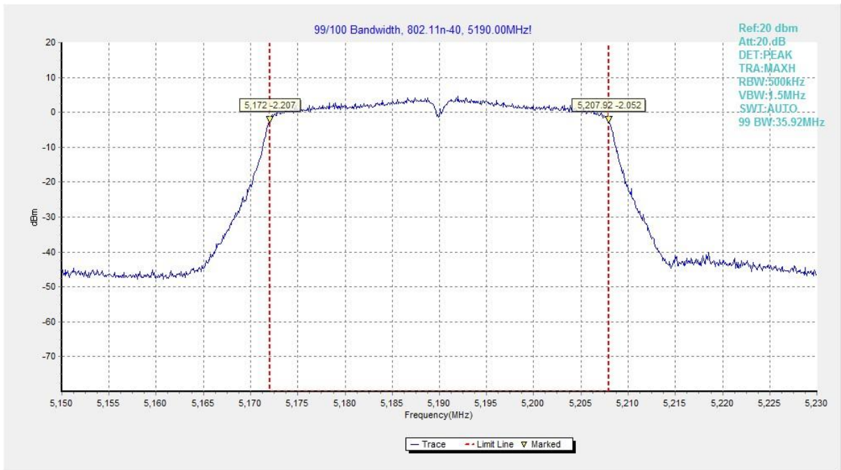
Fig. 39 99% Occupied Bandwidth (802.11n-HT40, 5190MHz)
