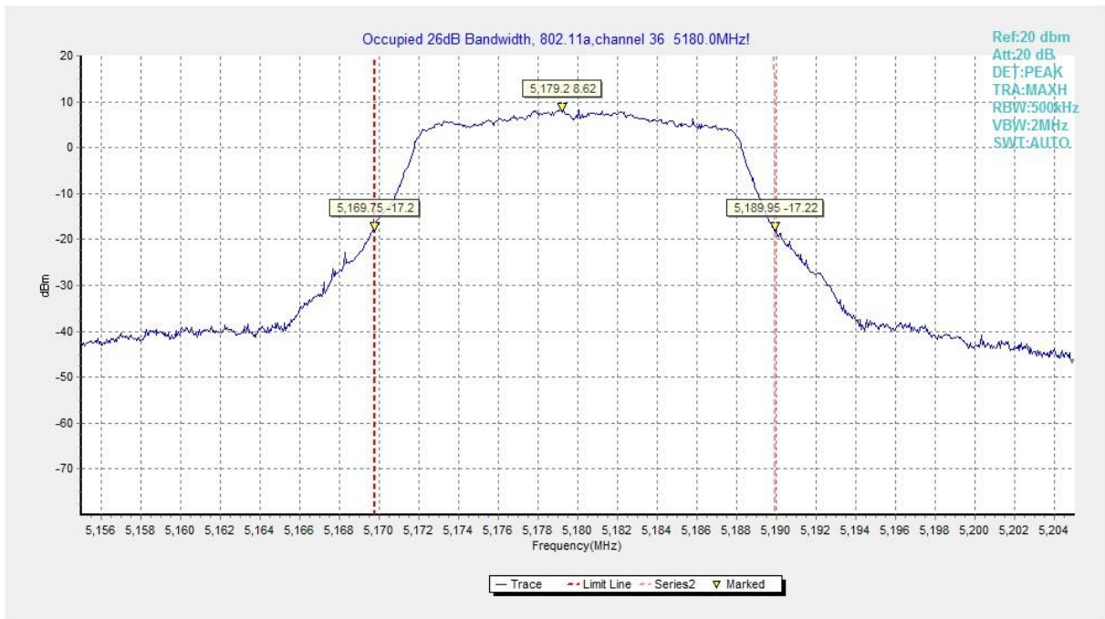
Fig. 1 Occupied 26dB Bandwidth (802.11a, 5180MHz)
