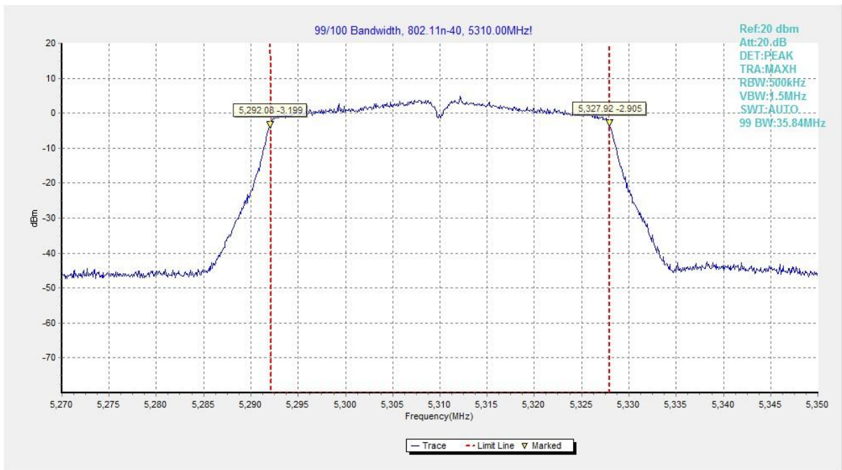
Fig. 42 99% Occupied Bandwidth (802.11n-HT40, 5310MHz)
