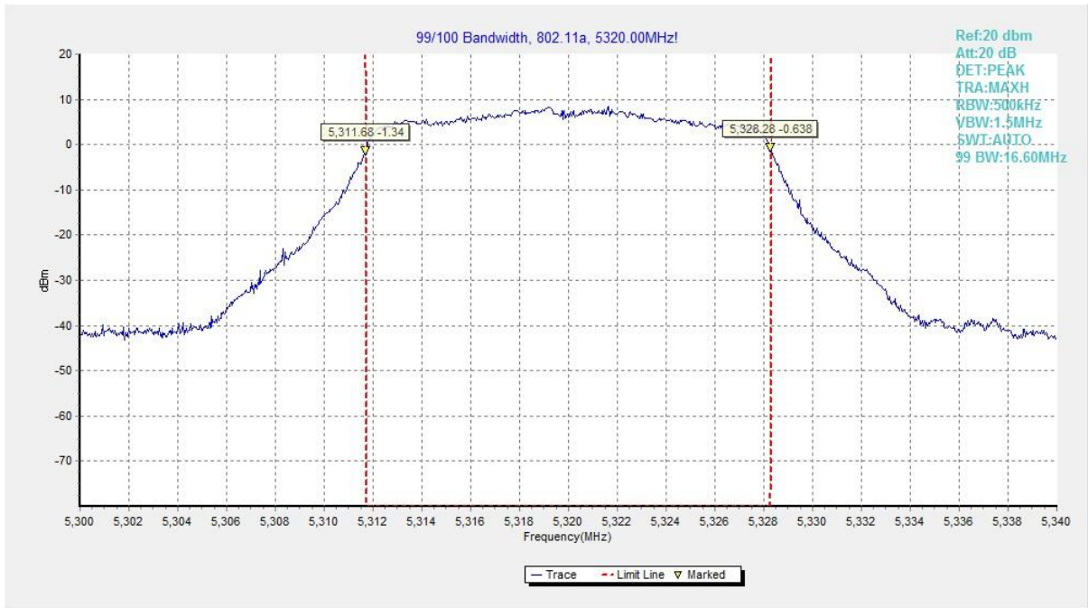
Fig. 32 99% Occupied Bandwidth (802.11a, 5320MHz)
