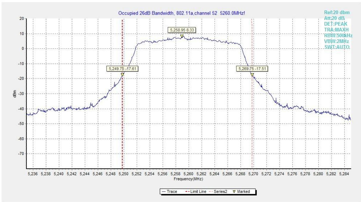
Fig. 4 Occupied 26dB Bandwidth (802.11a, 5260MHz)
