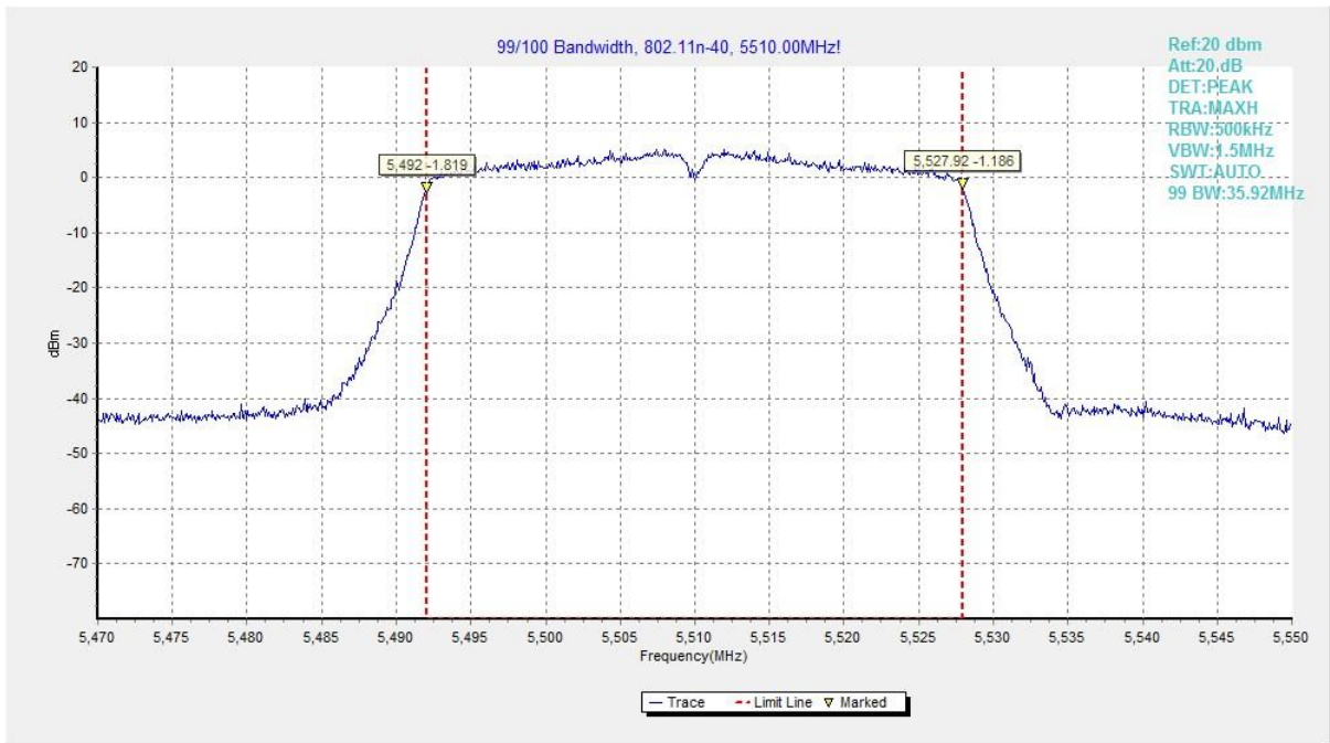
Fig. 43 99% Occupied Bandwidth (802.11n-HT40, 5510MHz)
