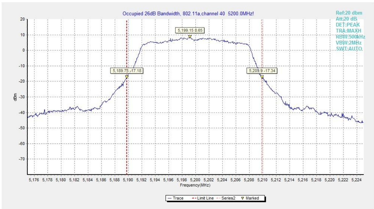
Fig. 2 Occupied 26dB Bandwidth (802.11a, 5200MHz)
