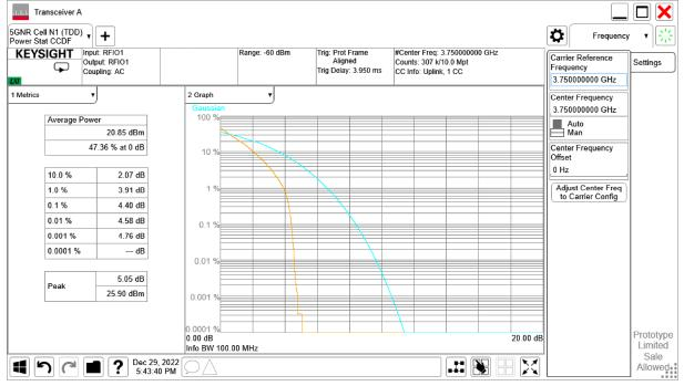
n78H, 100MHz Bandwidth, DFT-s-QPSK (PAPR)
