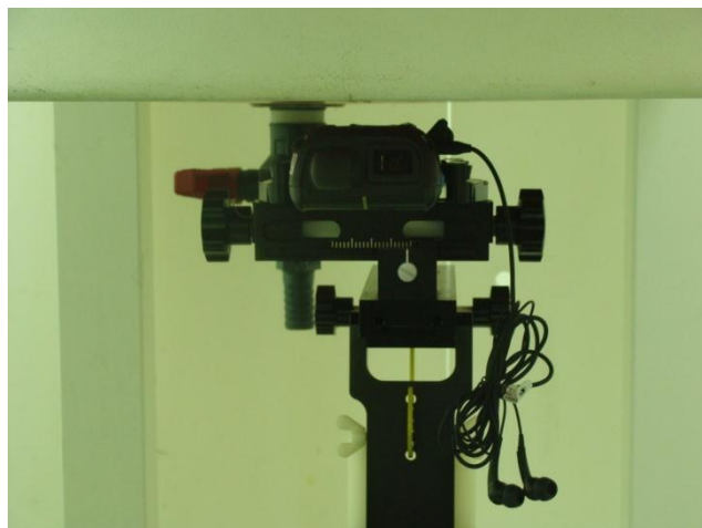
Back of the DUT with Phantom 1.5 cm Gap with Battery 1
