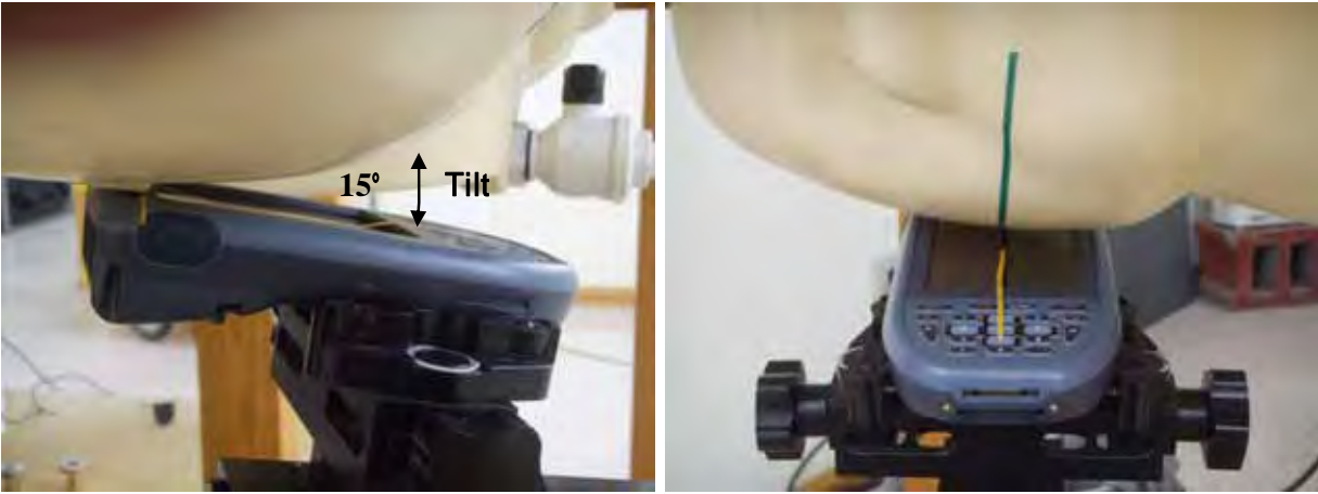
Fig.4 Right Head Section / Ear-Tilt Position(15°)
