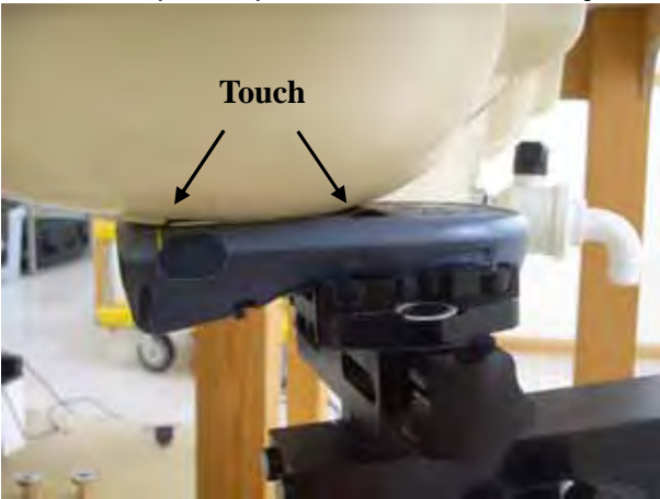
Fig.3 Right Head Section / Cheek-Touch Position
