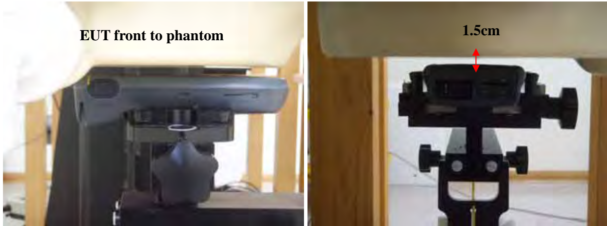
Fig.7 Body worn- EUT front to flat phantom and distance between flat phantom and mobile phone is 1.5 cm
