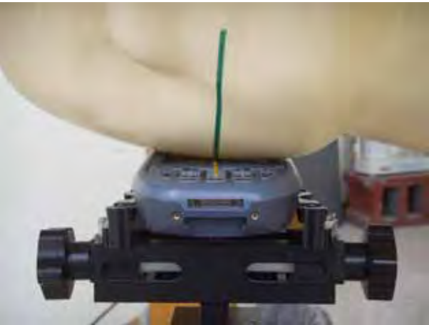
Fig.3 Right Head Section / Cheek-Touch Position
