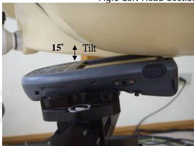
Fig.6 Left Head Section / Ear-Tilt Position(15°)
