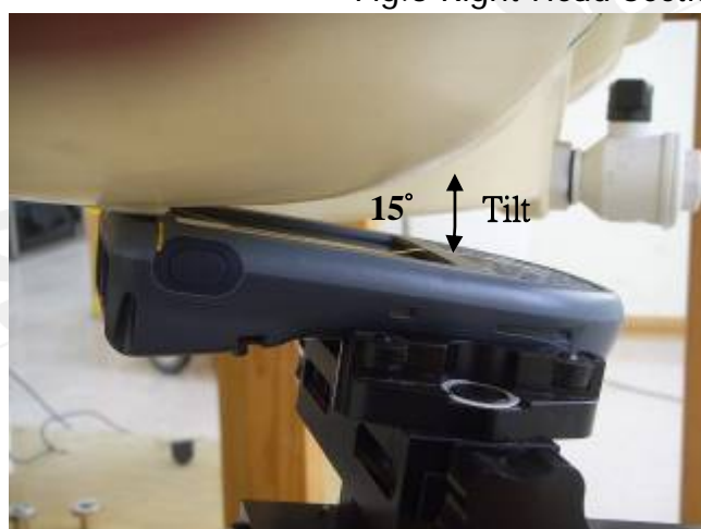
Fig.4 Right Head Section / Ear-Tilt Position(15°)
