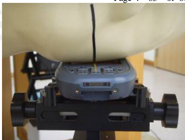
Fig.5 Left Head Section / Cheek-Touch Position
