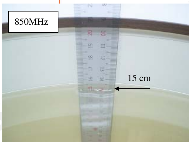
Fig.2.3 Photograph of the Tissue Simulant Fluid liquid depth 15cm for Flat (Body)
