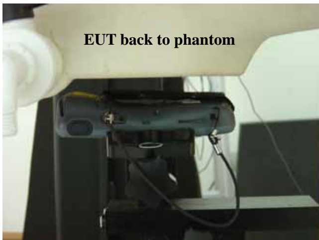
Fig.3 Body worn- EUT back to flat phantom and distance between flat phantom and mobile phone is 1.5 cm
