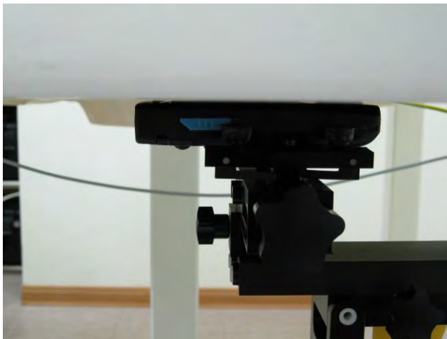
Fig.3 EUT front to flat phantom
