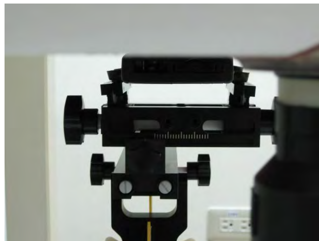
Fig.4 EUT back to flat phantom
