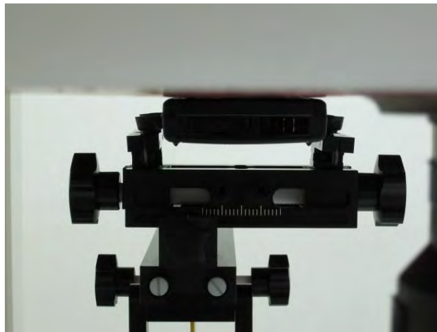
Fig.3 EUT front to flat phantom
