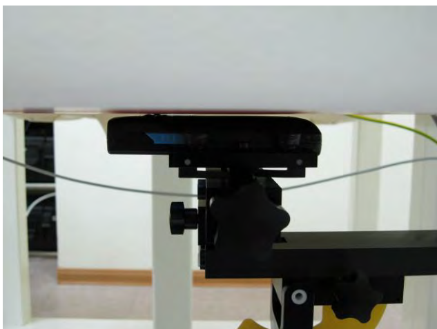
Fig.4 EUT back to flat phantom
