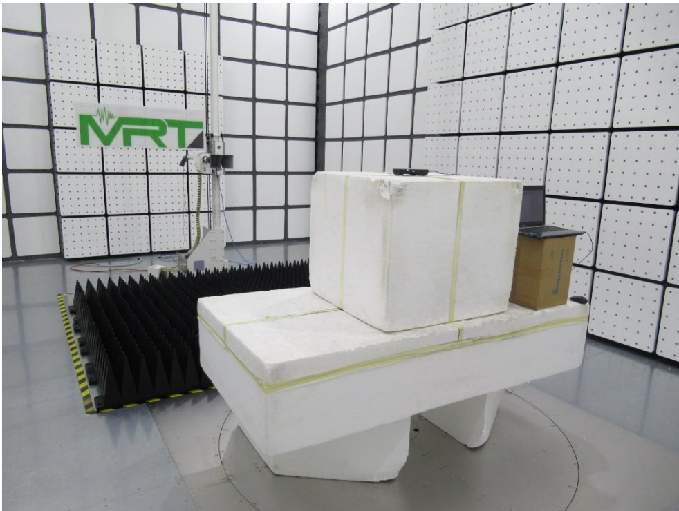
Description: Radiated Emission Test Setup for 1GHz~18GHz
