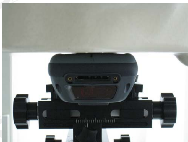
Fig.3 Front side of EUT is paralleled with flat phantom, separating 0cm between the back of the EUT and the flat phantom.
