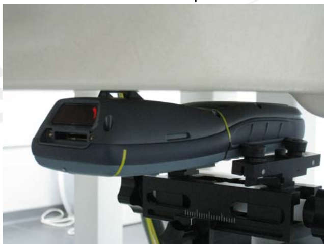
Fig.4 Back side of EUT is paralleled with flat phantom, separating 0cm between the back of the EUT and the flat phantom.
