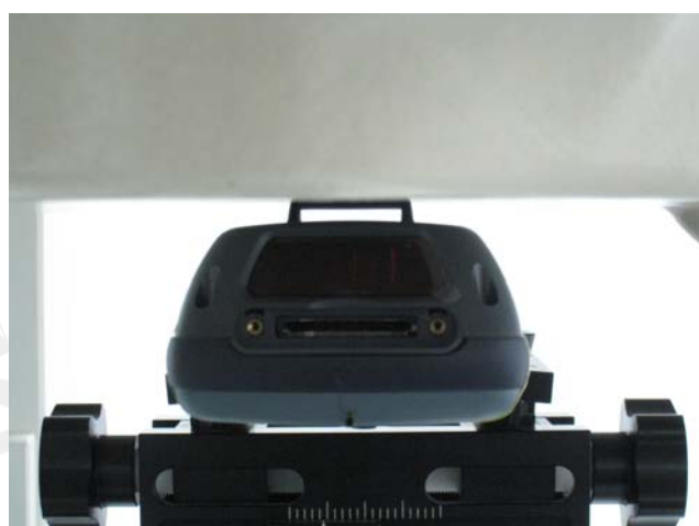
Fig.4 Back side of EUT is paralleled with flat phantom, separating 0cm between the back of the EUT and the flat phantom.
