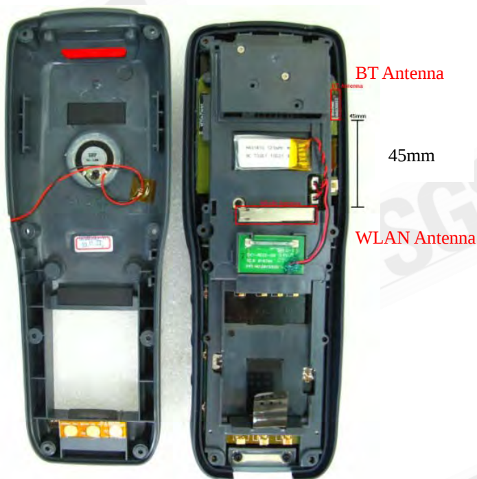
Fig.5 Antenna position & distance
