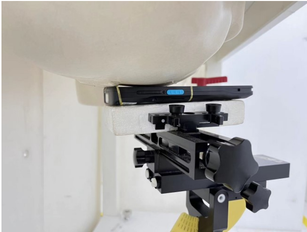
Right Cheek, Test Separation 0 mm
