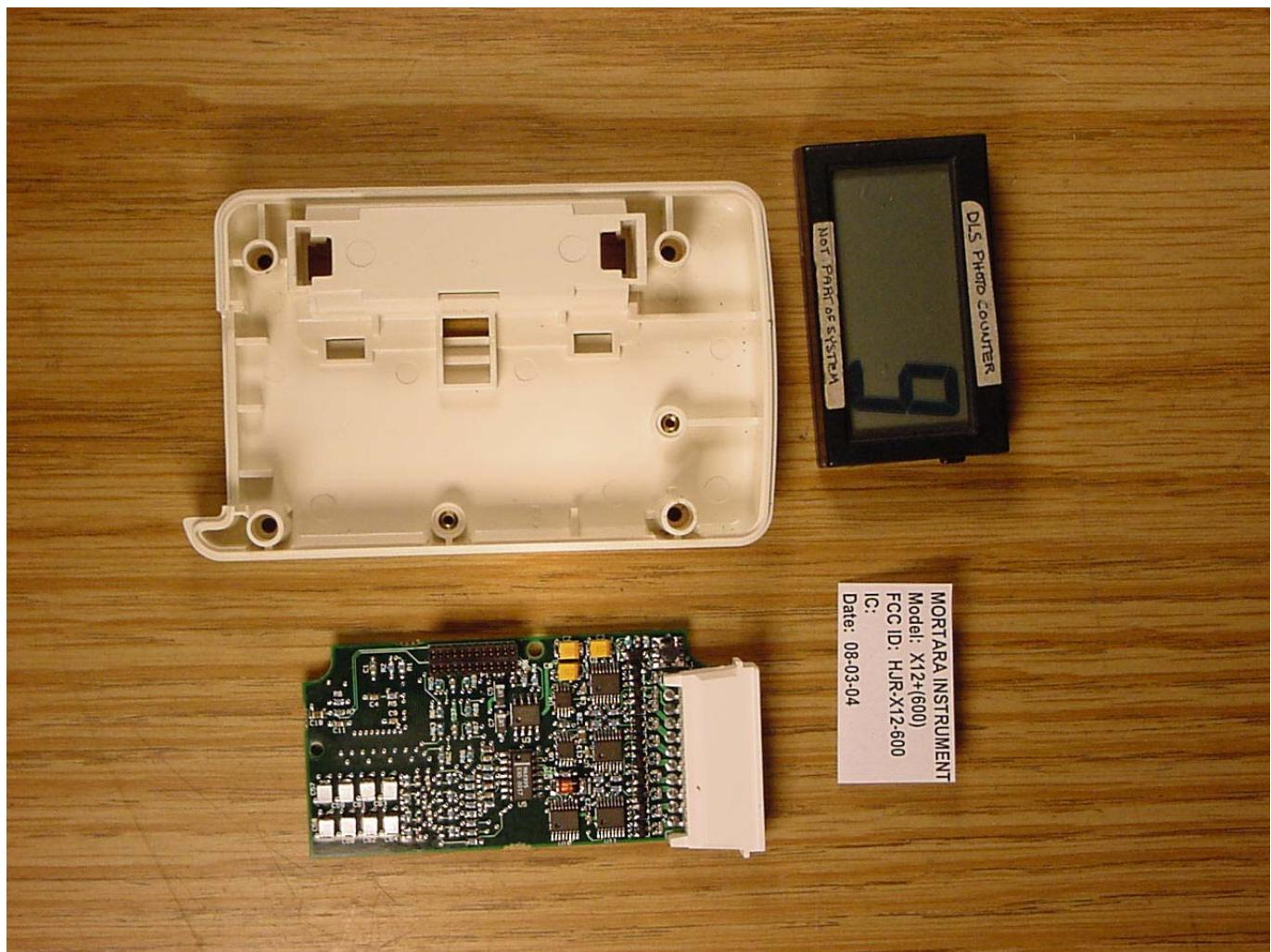
ECG FRONT END CARD REMOVED
