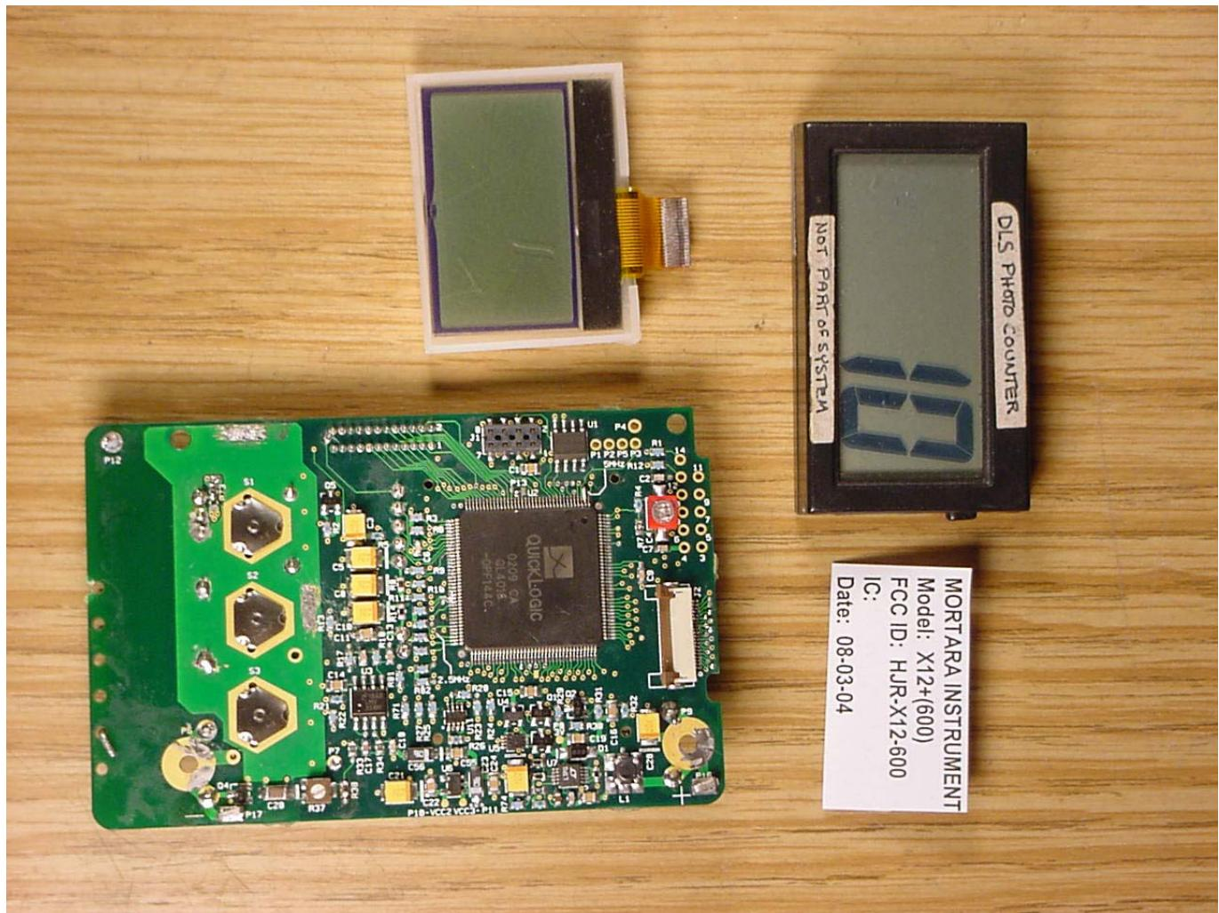
TRANSMIT CARD WITH LCD REMOVED
