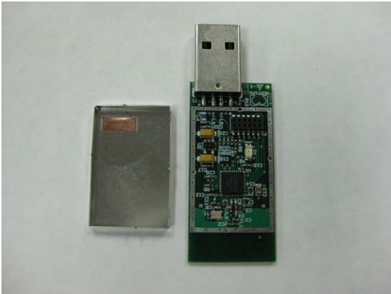
Open for Inspection – RF Section
