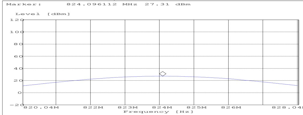
Mid channel 383 EIRP = 27.12dBm, ERP = 24.97 dBm
