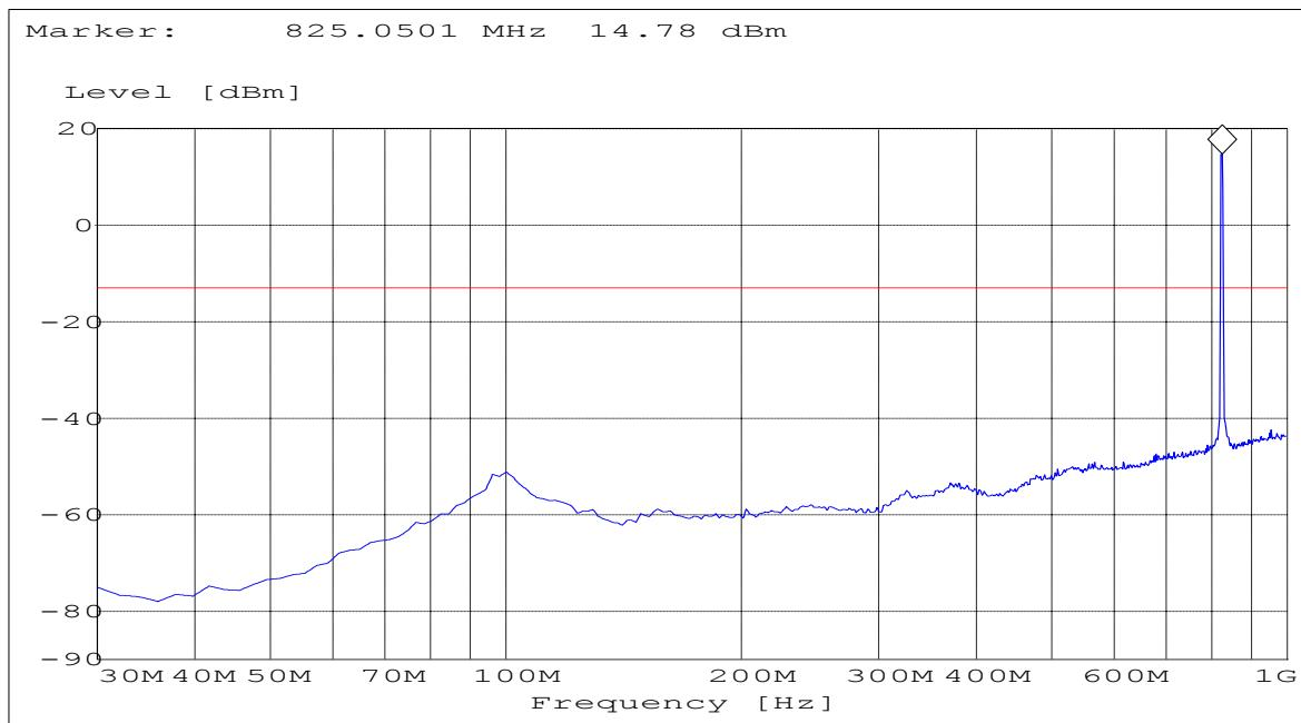
Note: The peak above the limit line is the carrier freq. at ch-991.
