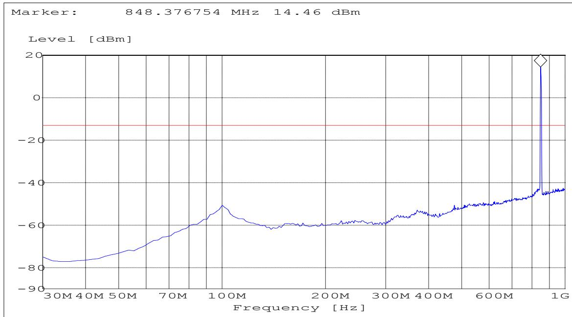
Note: The peak above the limit line is the carrier freq. at ch-799.
