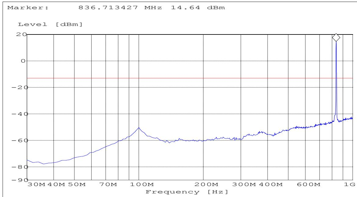
Note: The peak above the limit line is the carrier freq. at ch-383.
