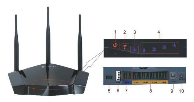
**1.Power LED** Off: powered off On: powered on
