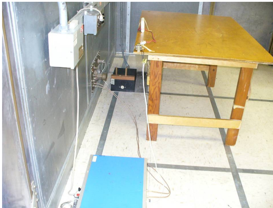
Photographs 1 & 2: Conducted Emission Setup
